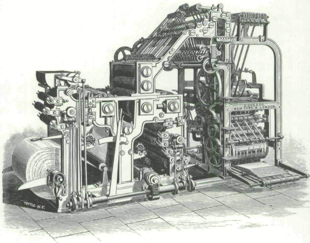
PLATE XXIII.—The 'Presto' Patented Stereotype Perfecting Printing Machine
