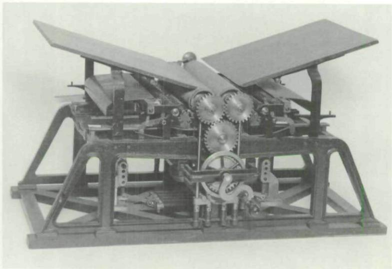
PLATE III.—Patent Office model of the 'Pony' Double Cylinder Press.
