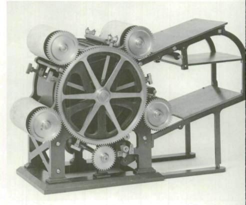
PLATE VI.—Patent Office model of the Type-Revolving Press. (Courtesy of the Smithsonian Institution.)
