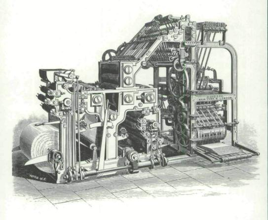
PLATE XXIII.—The 'Presto' Patented Stereotype Perfecting Printing Machine (Inland Printer, February, 1885).
